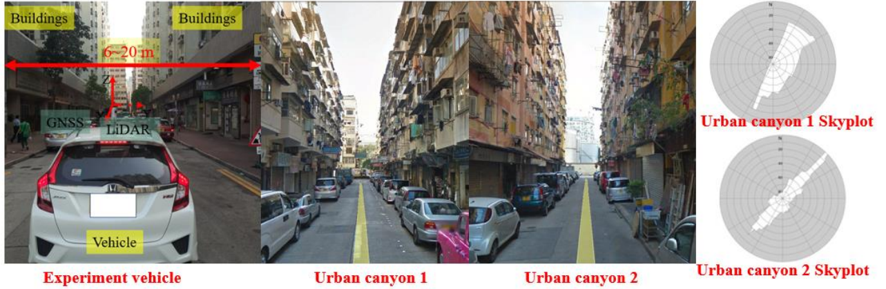
Fig. 7. The sensors setup of the vehicle and tested environment: GNSS and LiDAR sensors are installed on the top of the vehicle shown in the left side of the figure. The two tested urban scenarios are shown in the middle of the figures. The Skyplot of the two experiments is shown in the right side of the figure.
